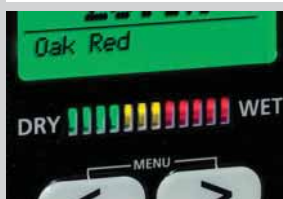
12-position wet/dry LED indicator
